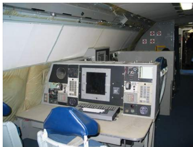
Battle Staff Position on Looking Glass Aircraft PD-3500 Plasma Display Terminal (Photo from SAC ACCA files-Photographer unknown)
